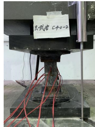
Figure 1-4 Field device diagram of axial compression test
