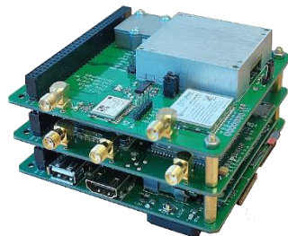
Figure 1. CoDRIVE on-board unit (OBU) for positioning, communication and processing
