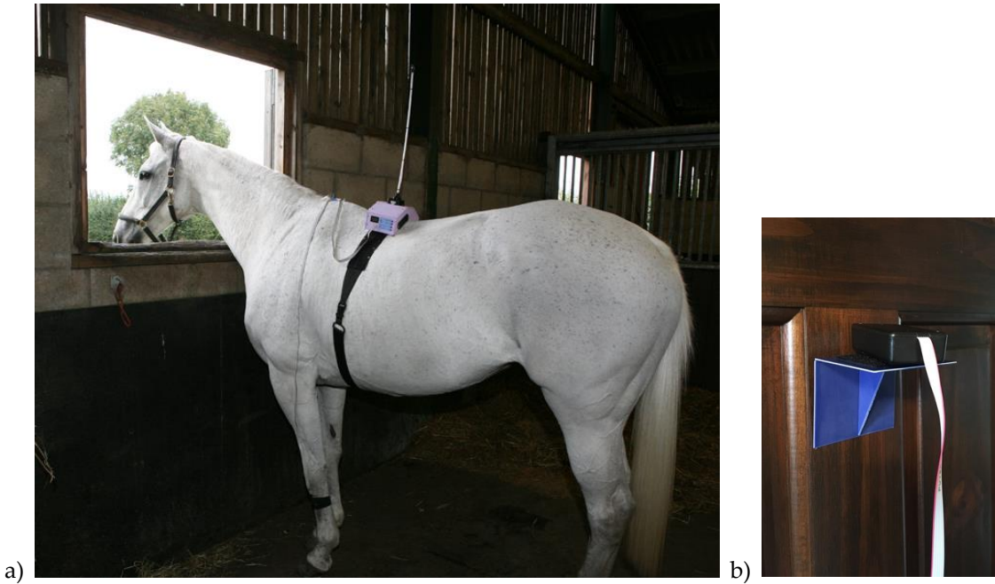
Figure 5. a) Thermal unit with receiver mounted on aerial on a horse’s back. b) Transmitter placed high on stable wall
