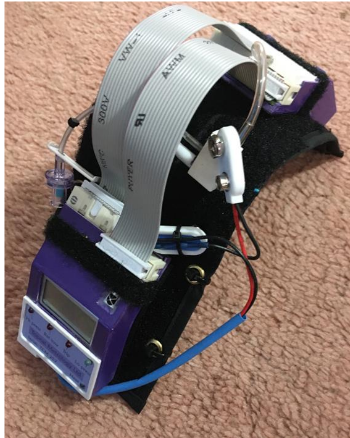
Figure 2. Remote controlled cat thermal band with cover removed.
