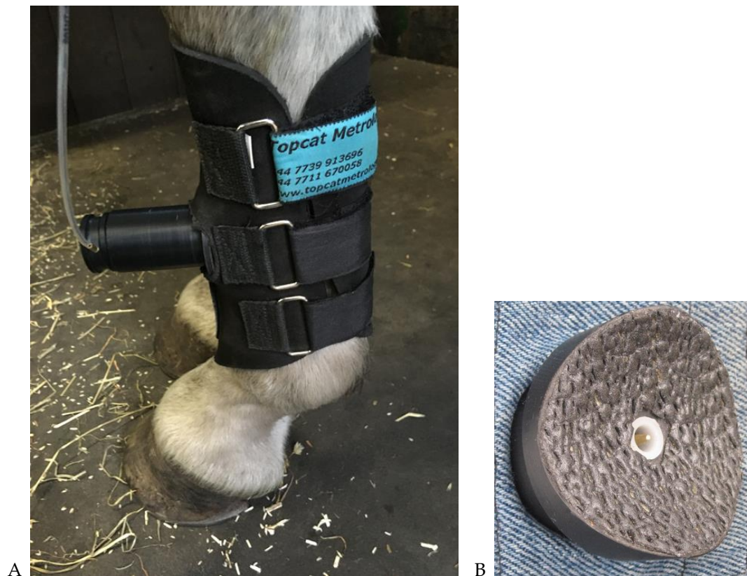
Figure 7. Pneumatic actuator. A: secured with boot and carefully tensioned band on forelimb of a horse standing free in its stall. B: the leg side of the actuator showing probe tip in resting position
