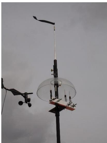
**Figure 1.** SPME sampler stand with 4 field SPME fibers in place.
