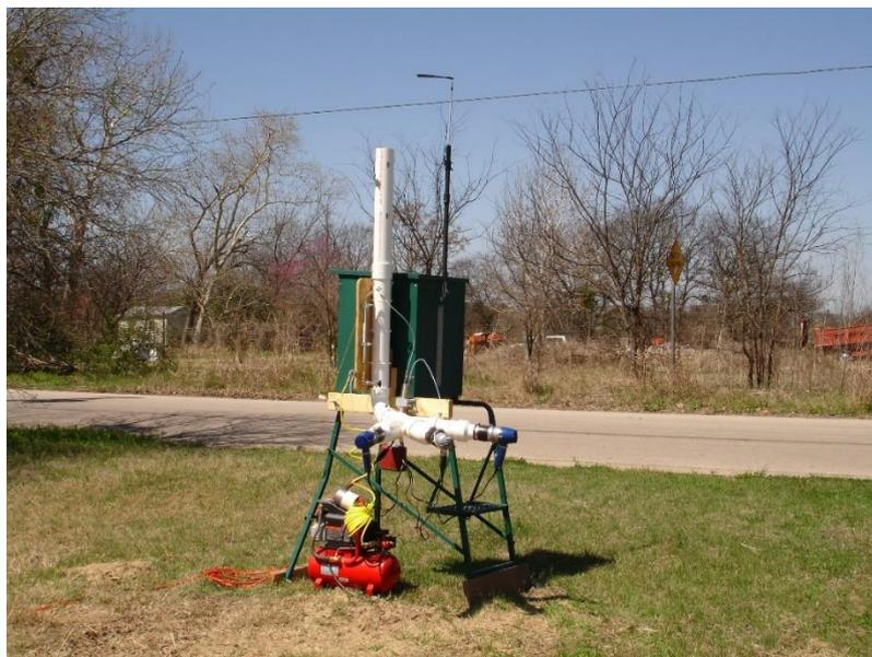
**Figure 5.** First-generation prototype scale-model transient odor event simulator.
