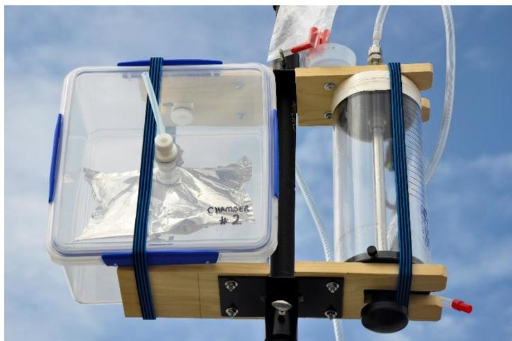
**Figure 3.** Second generation prototype grab sampling assembly: Close-up of syringe and sampling bag chamber 'cartridge' assemblies.
