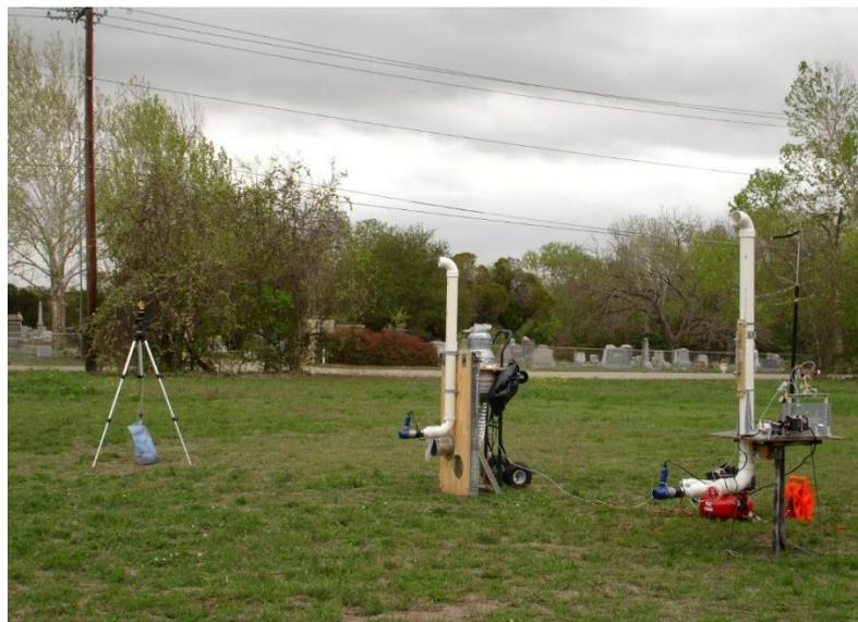
**Figure 7.** Integrated multiple point-source transient odor event generator systems. To the right are the two contrasting point-sources. To the left background is the tripod-mounted weather data logger.
