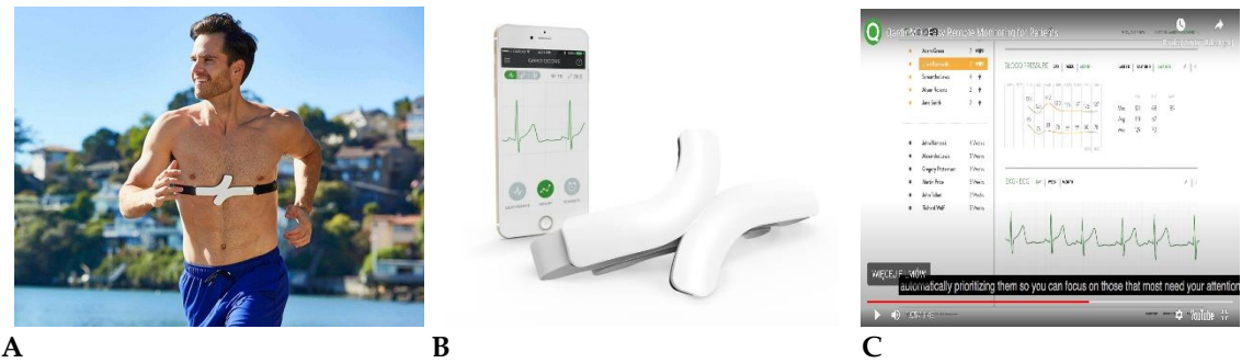
Figure 2. QardioMD ECG solution (QARDIO MD VSI sytem). (A) QardioCore ECG - chest strap with electrode. (B) Qardio mobile app ( ECG recording on iPhone ) and chest strap (QardioCore ECG) with electrode. (C) ECG recording on QardioMD remote monitoring web based portal.
