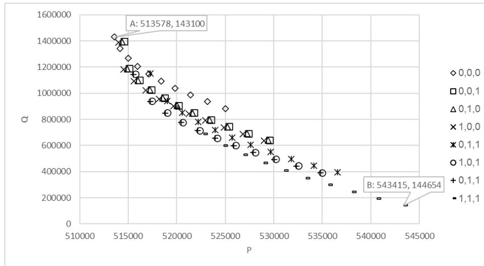
**Figure 3.** Calculated active power ( $P$ ) and reactive power ( $Q$ ) for all control points in the test feeder, with highlighted extreme points.
