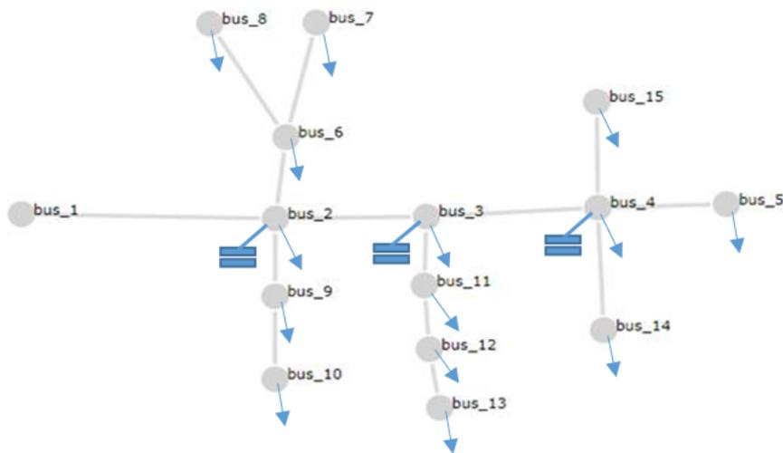
Figure 2. Schematic of the test feeder based on [32] with the addition of capacitor banks.
