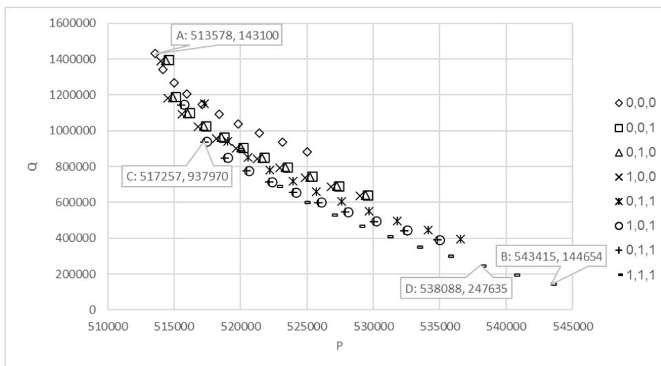
**Figure 5.** Calculated active power (P) and reactive power (Q) for all control points in the test feeder, with highlighted points of interest.
