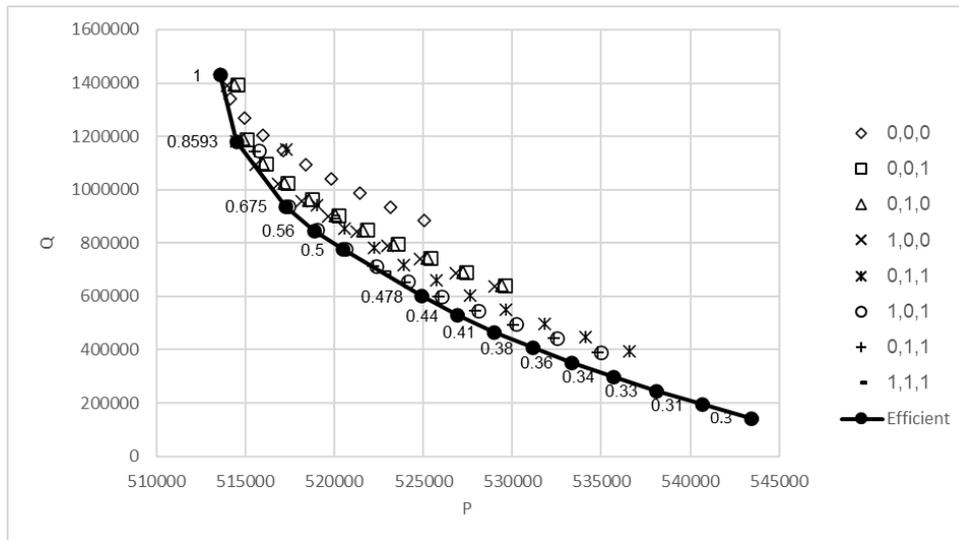
**Figure 4.** Active power (P) and reactive power (Q) on test feeder with efficient curve highlighted and  $\alpha$  values.
