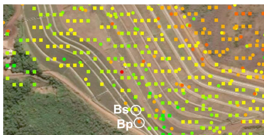
Figure 15. SBAS and PSI results combined and the locations of Bs and Bp points on the dam bottom; SBAS MPs are represented by square symbols and PSI MPs by circles.
