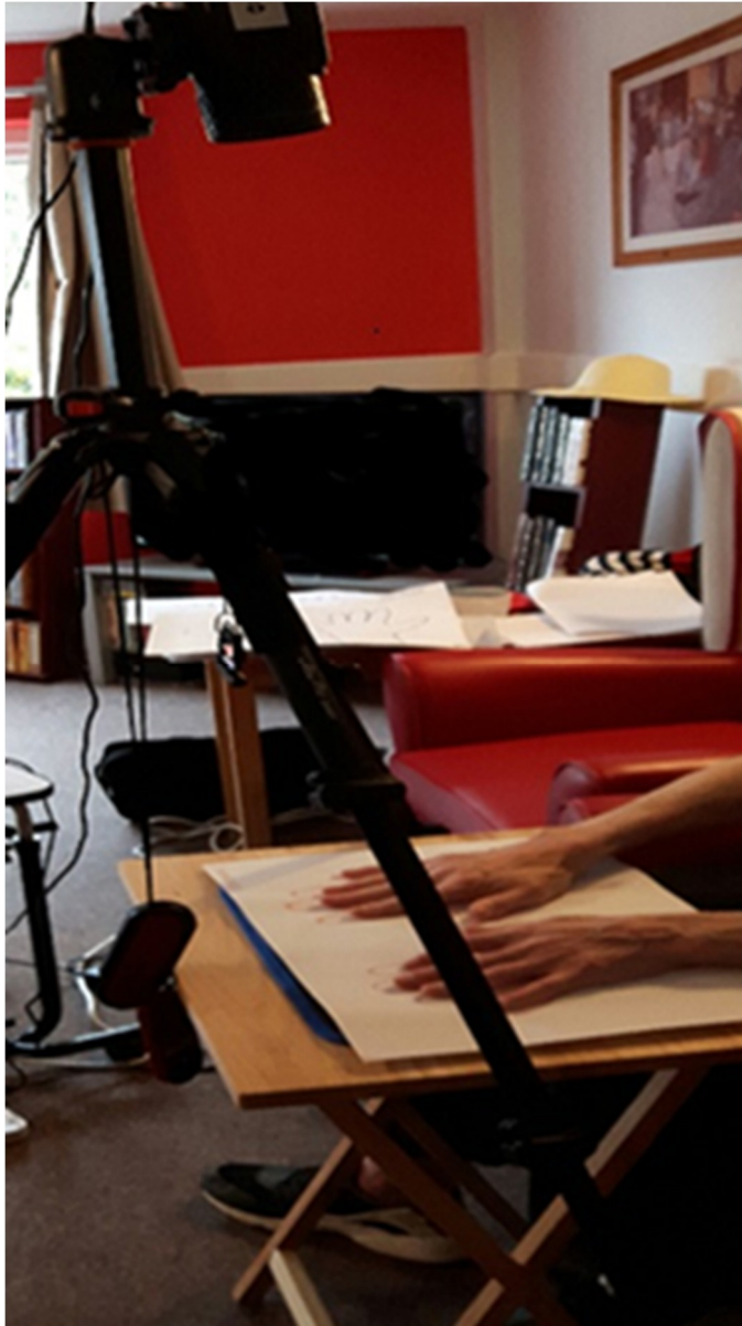
Fig 1: Long wave infrared imaging detector mounted on tripod. Figure shows the participant during imaging with hands positioned upon a paper 'hand template' overlying an insulated tile. The portable table was used throughout the study to ensure consistency of the imaging set-up .
