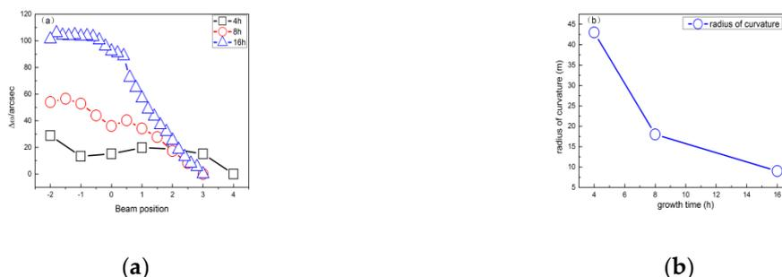
**Figure 4.** (a) Relative position  $\omega(\Delta\omega 400)$  as a function of x-ray beam position on diamond plane for different growth times. (b) Radius of curvature as a function of growth time.
