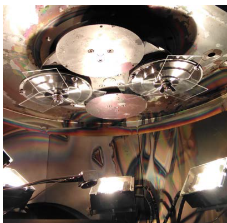
Figure 5. E-beam deposition system: glass substrates mounted on the rotating planetary
