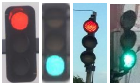
Figure 16. From left to right: examples of green and red traffic lights used in training, examples of green and red traffic lights obtained by the TLR device and used in tests.
