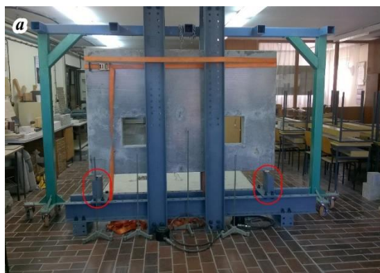
Figure 13. Steel frame for testing reinforced concrete members: a) frame appearance and b) geometric characteristics.
