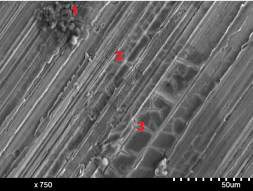
Figure 17: SEM micrograph of oxidised steel
