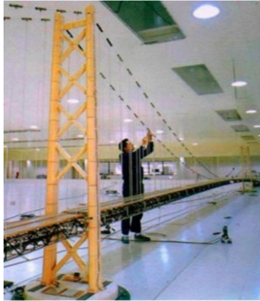
Figure 4. Akashi Kaikyo Bridge model in a wind tunnel [31].
