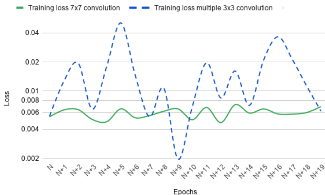
Figure 2. Training loss of two different type convolution networks. The training loss was extracted from a 20 epoch window while training. N depicts the start of the window and the loss were plotted for each epoch. Training loss of convolution network with two different kernel size ( 3 \times 3 and 7 \times 7 ) is plotted.
