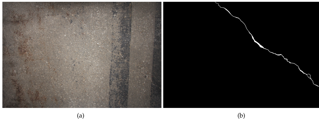
Figure 8. (a) Sample crack image and (b) annotated image from the Illinois Bridge data-set.
