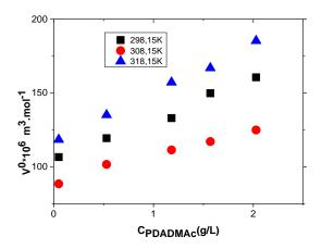
Fig. 4. Plot of  $V_{\phi}^{0}$  for surfactant SDS in aqueous solutions of PDADMAc at different temperatures.
