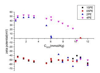
Fig.6.Zeta potential of SDS–PDADMAc samples as a function of the molality of surfactant.  $\triangle 1.5g.L^{-1}$ ,  $\bigtriangledown 2g.L^{-1}$ ,  $\bigcirc 0.5g.L^{-1}$  and  $\Box 1g.L^{-1}$  of PDADMAc
