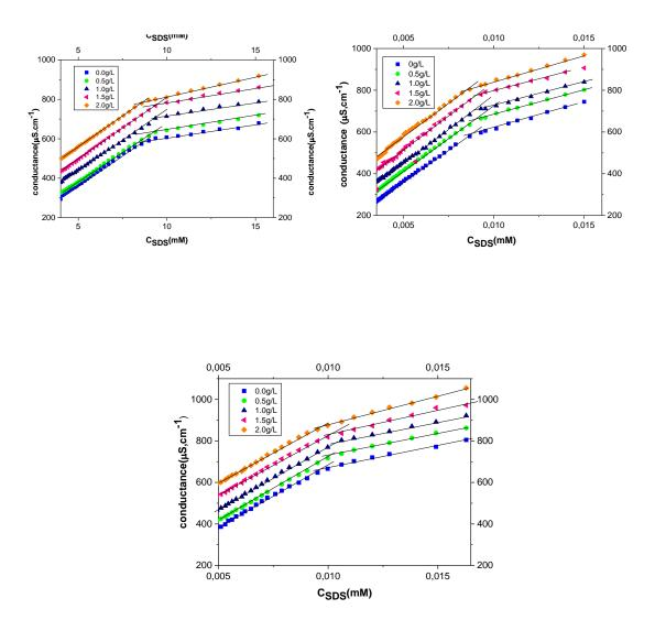
Fig. 1. Specific conductance ( $\kappa$ ) of aqueous SDS solutions in the presence of different concentrations of PDADMAc at temperatures (a) 298.15 K; (b) 308.15 K; (c) 318.15 K.
