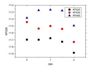
Fig. 5. The variation in limiting apparent adiabatic compressibility,  $K_{\phi}^{0}$  as a function of concentration of PDADMAc at different temperatures.
