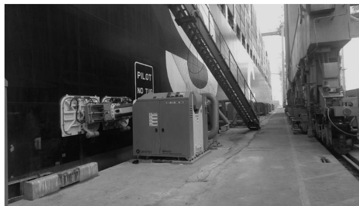
Fig. 1. Automatic Mooring System by vacuum cups in Salalah. Source: Cavotec
