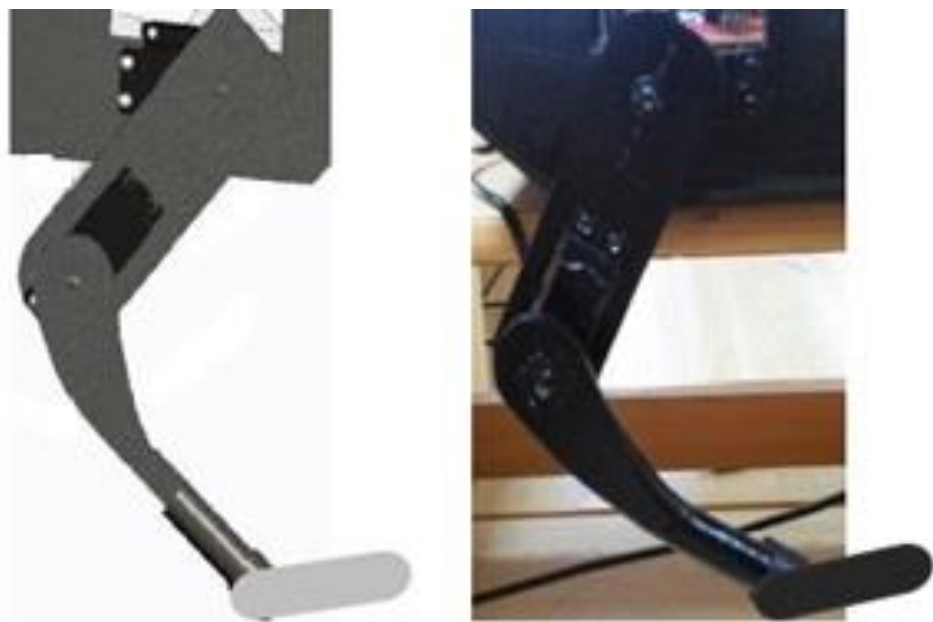
Figure 7 Single leg test configuration indicating the foot trajectory path (Left: simulation, right: real).
