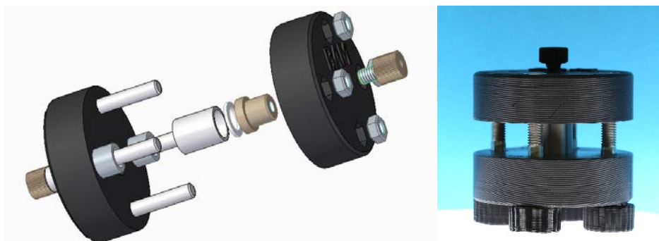
Figure S1. Engineering drawing of the additive-manufactured column holder (Solid Edge; Bettina Roeder, BAM) with custom 1/16" PEEK fittings and monolithic affinity column (left), and photo (Martin Paul, BAM) operational column ready to use (right).
