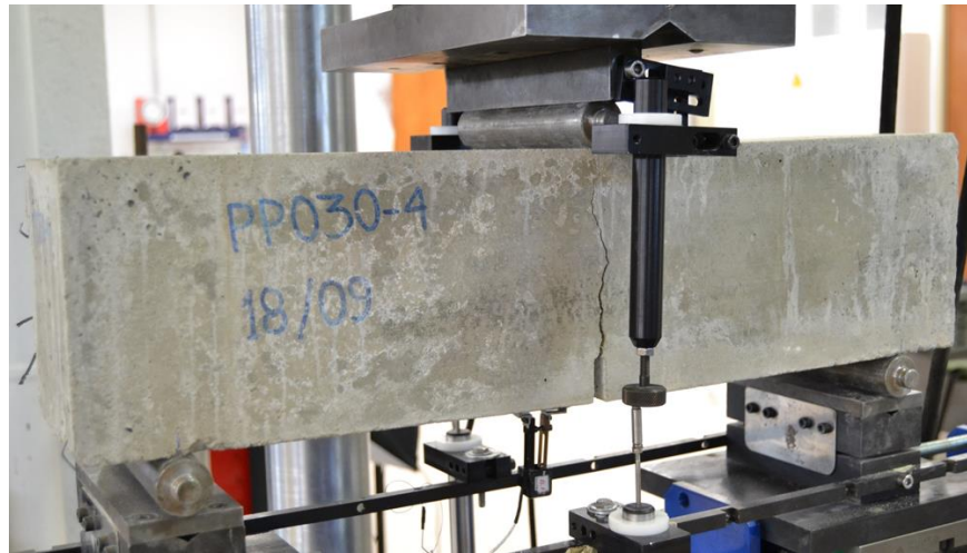
Figure 2. Three-point bending test.
