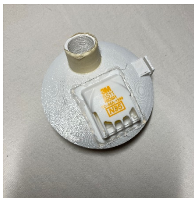
Figure 17. Apply tape to the nozzle to provide and air-tight fit to the hose.
