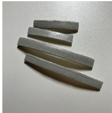
Figure 13. Weather-seal gasket, cut in half lengthwise.
