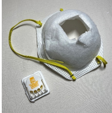
Figure 14. 3M Cool-Flow Exhalation Valve removed from mask.
