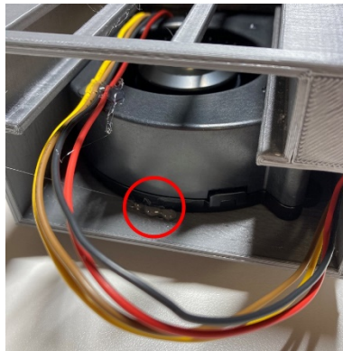
Figure 19. Glued fan in place (if necessary).
