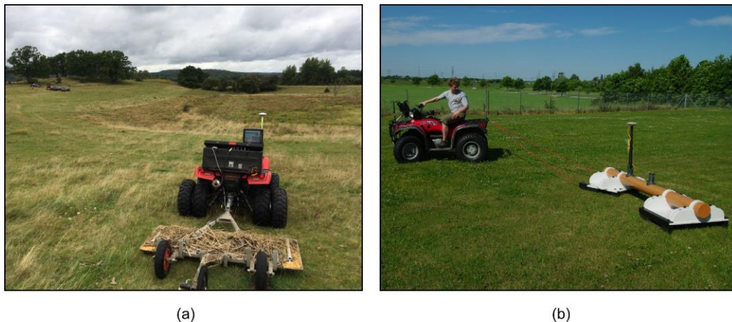
Figure 3. a) The 3D-GPR instrument and b) the DUALEM-21S sensor.
