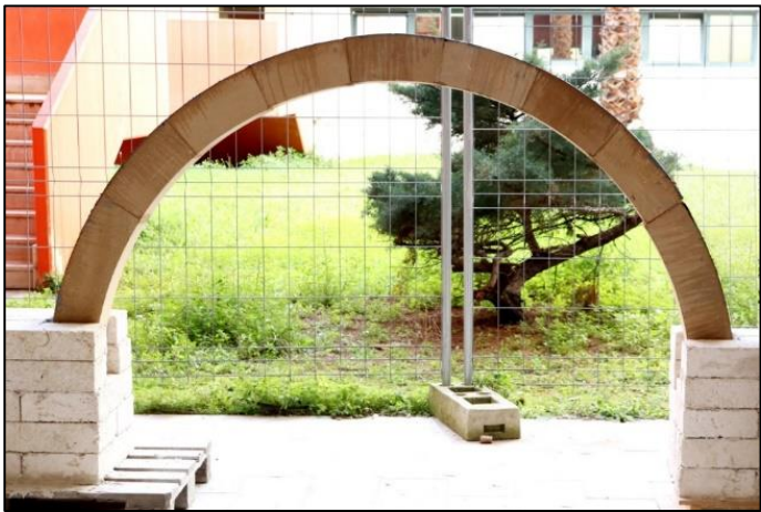
Figure 12. Placing of the HLA on the buttresses.
