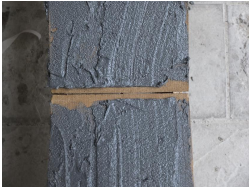
Detail of the free resin line.
