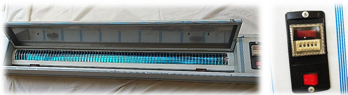
Figure.2. The used UV radiator having a 36W quartz UVC lamp, a manually programmable and on/off switch.
