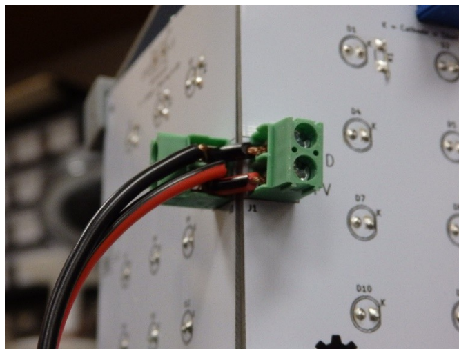
Figure 11. Two cables tapped into a terminal set for power flow from the supply
