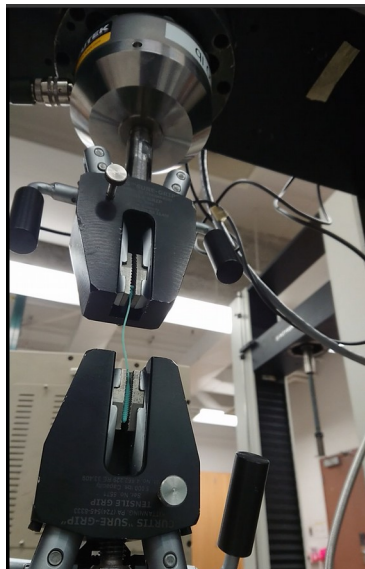
Figure 25. Mechanical testing of swabs with an Instron 4206.
