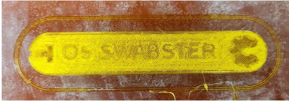
Figure 21. As printed version of handle on a Lulzbot Taz 6 print bed
