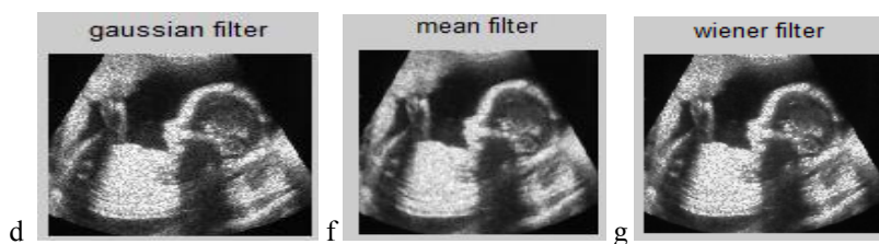
Fig. 7. Result of filtering for eliminating Speckle noise from Ultrasound image
