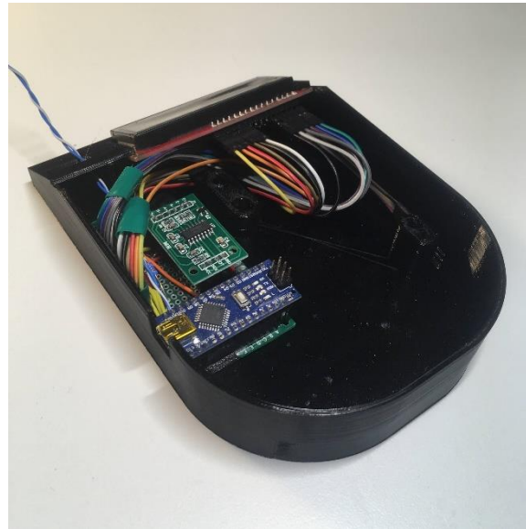
Figure 6. The LCD is held in place by two locators behind the slot for the screen. Its wires are tucked under a plastic wire manager attached to the TAL220 boss, then connected to the circuit board.
