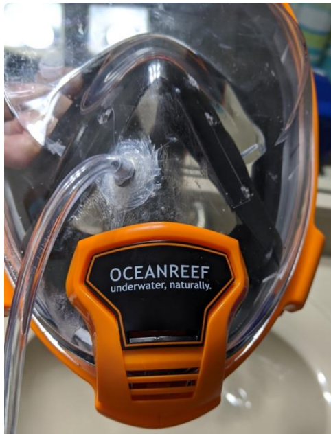
Figure 2. Metal grommet covered with silicone on its outside and inside flat surfaces and extending beyond the grommet's edge to eliminate potential air leaks. The PortaCount's testing clear tube was secured with superglue.
