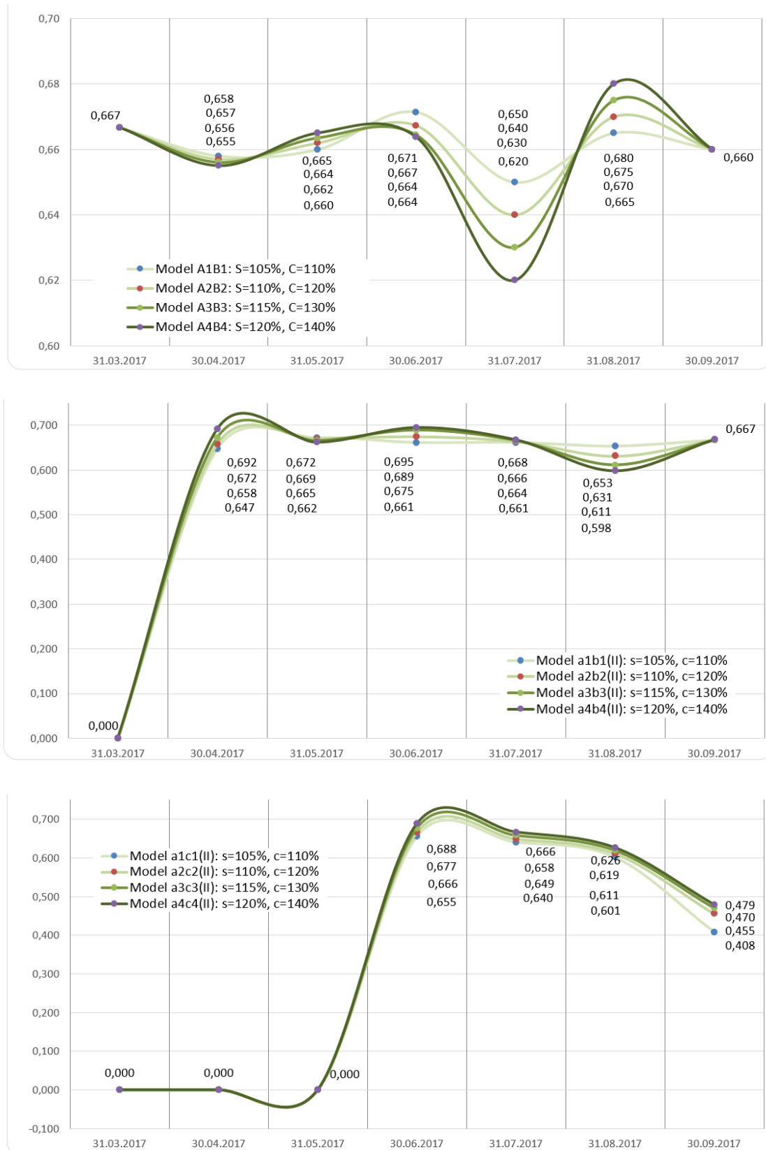
Figure 5. Monitoring indicator charts in the assumed financial liquidity due to arising variances from planned costs (T/C) in models with a gradually increasing time and cost variance - in the implementation methods according to (from above): steady, parallel, sequence execution of works. Source: [17]
