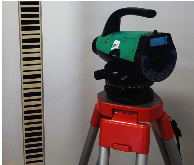
Figure 1. Example of a digital level – bar-code staff system [45].
