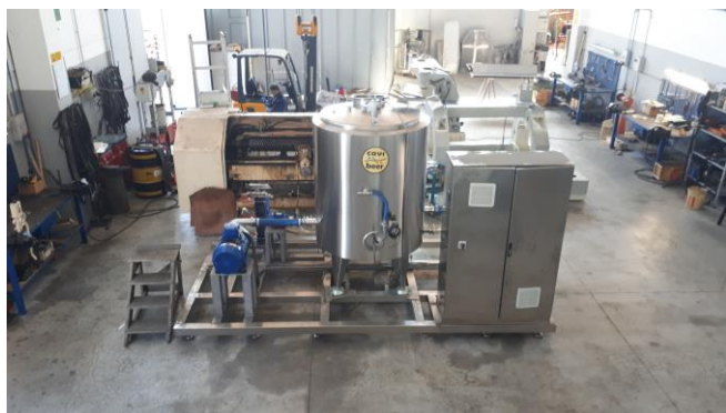
Figure 1. Available HC-based extraction plant at the GBL S.r.l. mechanical workshop, Italy
