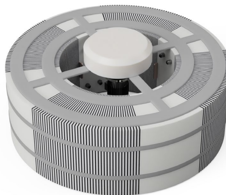
Figure 6. Rendering of 4 x 40 toroidal redox flow cell stack concept incorporating auxiliary plant (motor and pumps) capped and centrally mounted internally.
