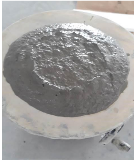
Figure 3. Flow of cement paste containing carbon fiber.
