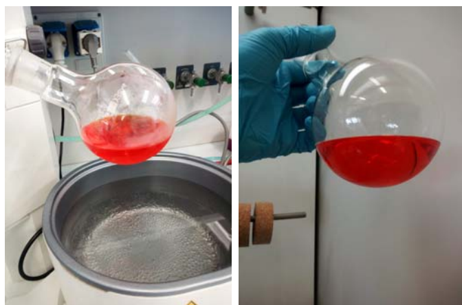
Figure 2. The extract from Parapenaeus longirostris carapace in limonene prior to evaporation of the biosolvent.
