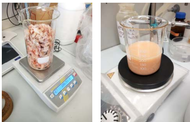
Figure 1. A sample of Parapenaeus longirostris carapace waste prior (left) and after homogenization with an electric blender (right).
