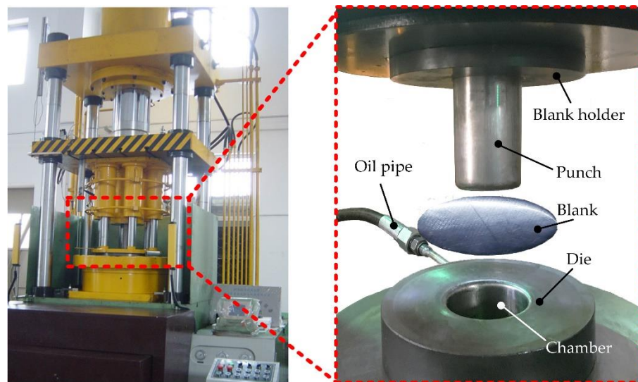
Figure 3. The die sets of hydrodynamic deep drawing process.
