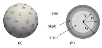
**Figure 2.** Head model with EEG electrodes: (a) PEC electrodes formed by triangles lying on the surface of the discretized 3-layer sphere, and (b) 3-layer spherical head model.
