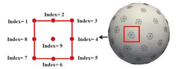
Figure 3. Indexes of the 9 possible positions of an electrodes.
