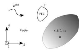
**Figure 1.** Description of the 3D scattering problem. The PEC parts are modeled by their boundary (i.e.  $\Gamma$ ) and the dielectric parts are modeled by their volume (i.e.  $\Omega$ ).
