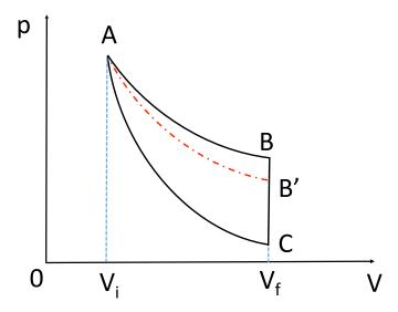
Figure 1: The ideal free expansion from state A to B can be represented by the isothermal process, AB, which is equivalent to an adiabatic expansion, AC, plus a constant volume process, CB. The Universe expands along the curve of the polytropic process, AB', infinitively close to the ideal isothermal process, AB. At different stages of universe evolution the polytropic index takes different values
