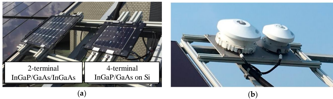
Figure 2. Measured 4T III-V/Si module and its solar cell structure: (a) Description of measured 4T III-V/Si module, 2 + 1 junctions (right) with comparison to the 2-terminal III-V 3-junction module. Note that the number of junctions is the same; (b) Spectro-radiometers installed at the University of Miyazaki [38].
