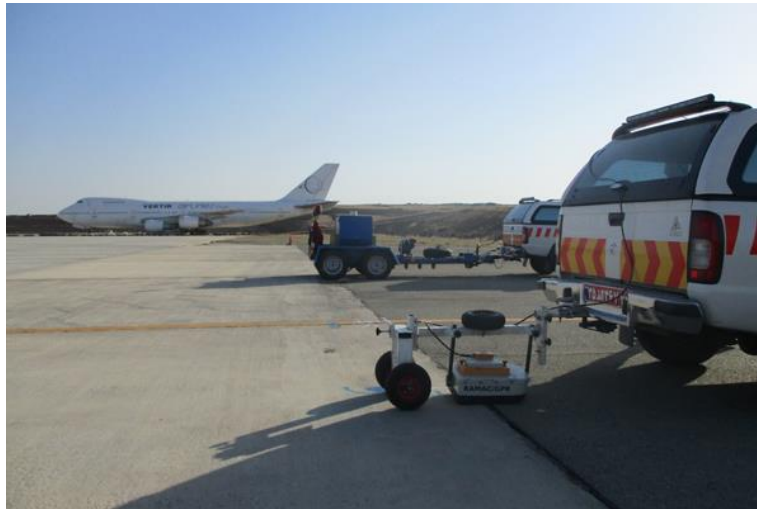
Fig. 1 GPR (closer machine) and HWD (farther machine) used in the study [41].
