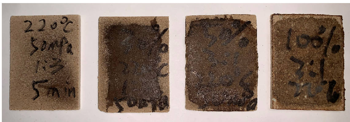
Figure 11. Samples of 50 MPa, 220 °C, 1:3 mixture proportion of concrete to wood, 5 min compaction duration, and different water content (10, 30, 50, and 100% from left to right)
