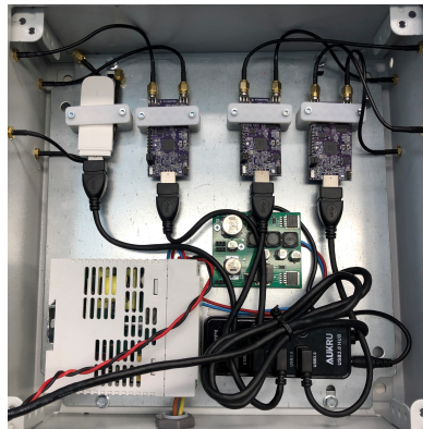
Figure 4. Gateway setup with 3xOpenMote-B boards, 1xRaspberry Pi 3B+ (not displayed) and a Huawei E3531 HSPA+ modem.
