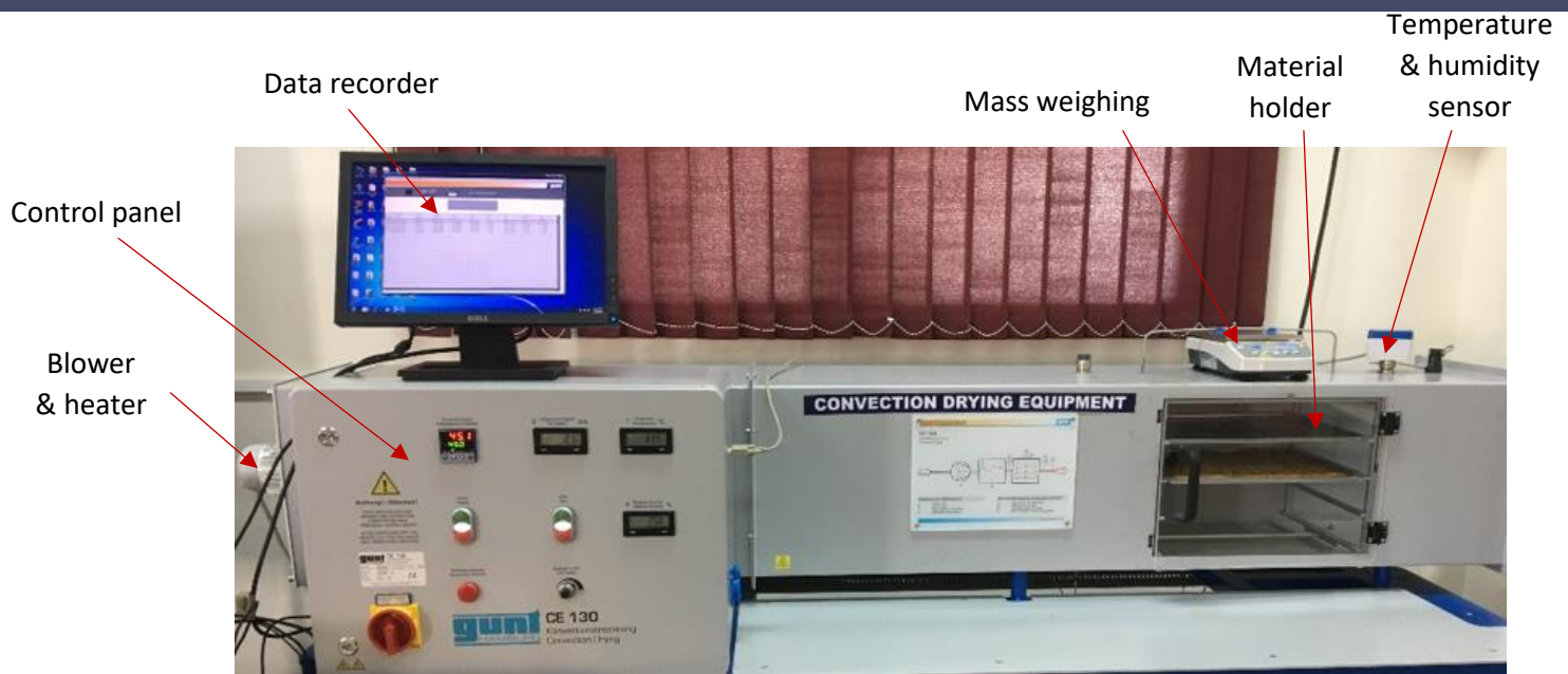
Figure 4. Laboratory scale forced convective tray dryer
