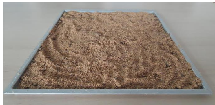
Figure 5. Uniform distribution of NCS sample on a tray area of 0.128 m 2
