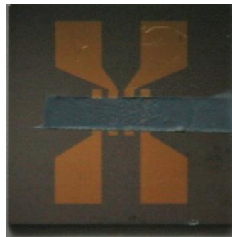
Figure 8: Gas sensing layer comprising \text{TiO}_2 nanoparticles and graphene flakes: photo of the sensor made by painting on a silicon substrate with four-point gold contacts.
