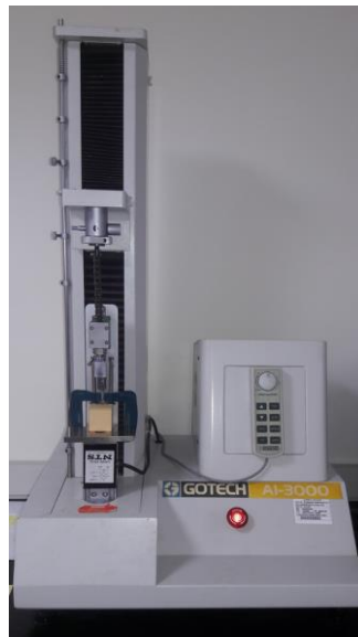
Figure 3. The material testing machine (GOTECH AI-3000, Taiwan) for the pullout strength (PS) test.
