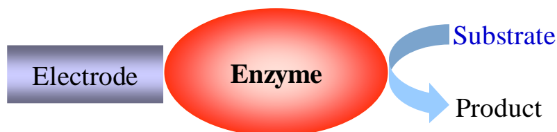
Figure 1. Schematic view of DET-type bioelectrocatalysis
