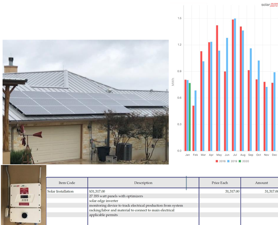
Figure 19. 10 kWh SolarEdge system (top left) with inverter (bottom left), power production (upper right), and acquisition costs (lower right)
