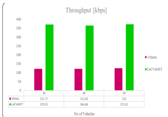
FIGURE XXX COMPARISON OF THE LAC-VANET PROPOSED SCHEME AND VMaSc MODEL IN TERM OF AVERAGE THROUGHPUT.
