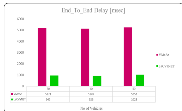
FIGURE LX COMPARISON OF THE LAC-VANET PROPOSED SCHEME AND VMaSc MODEL IN TERM OF DELAY.
