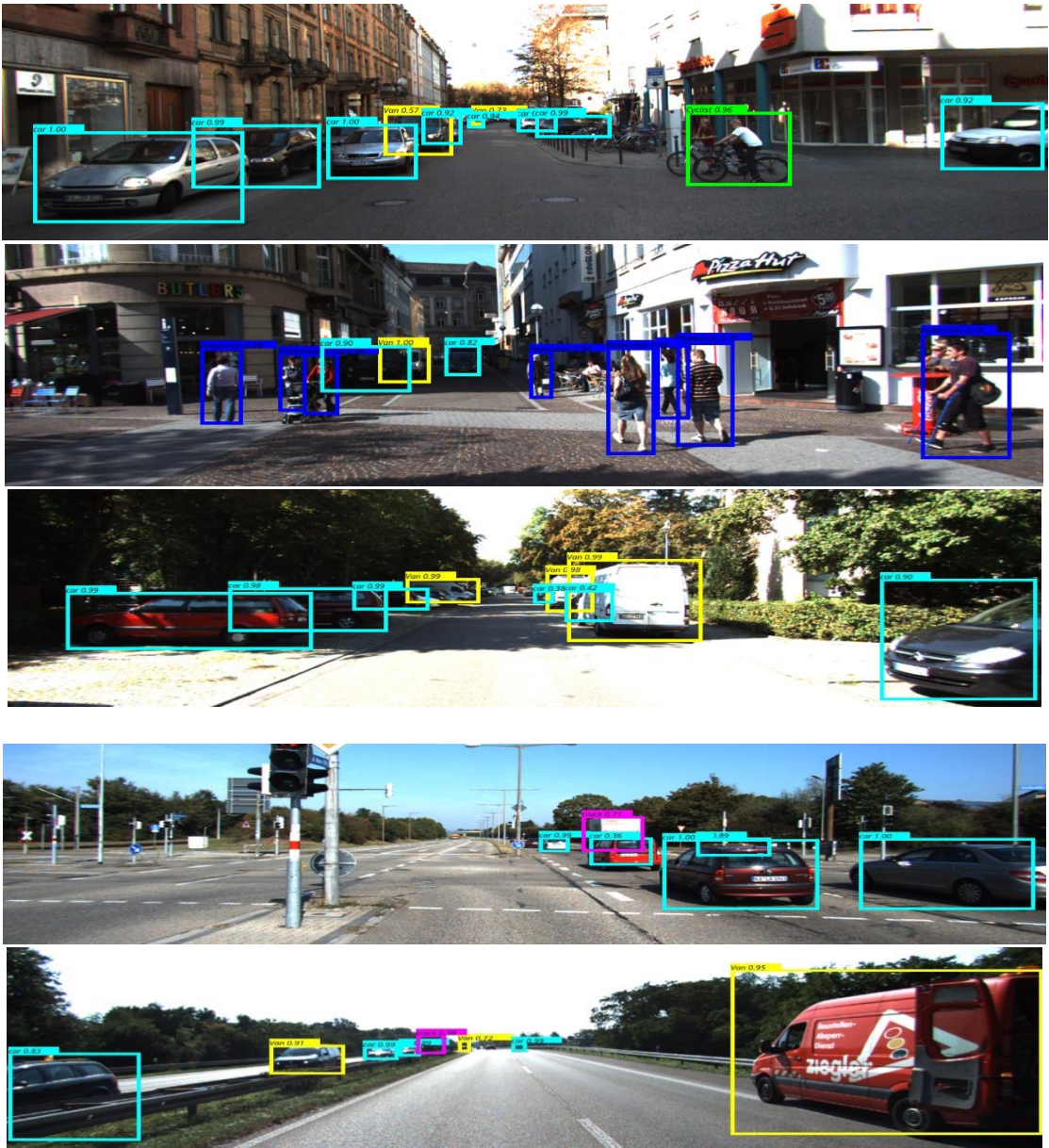
Figure 17: Obstacle detection has also been done using the YOLOv3 algorithm on the images obtained from real driving
