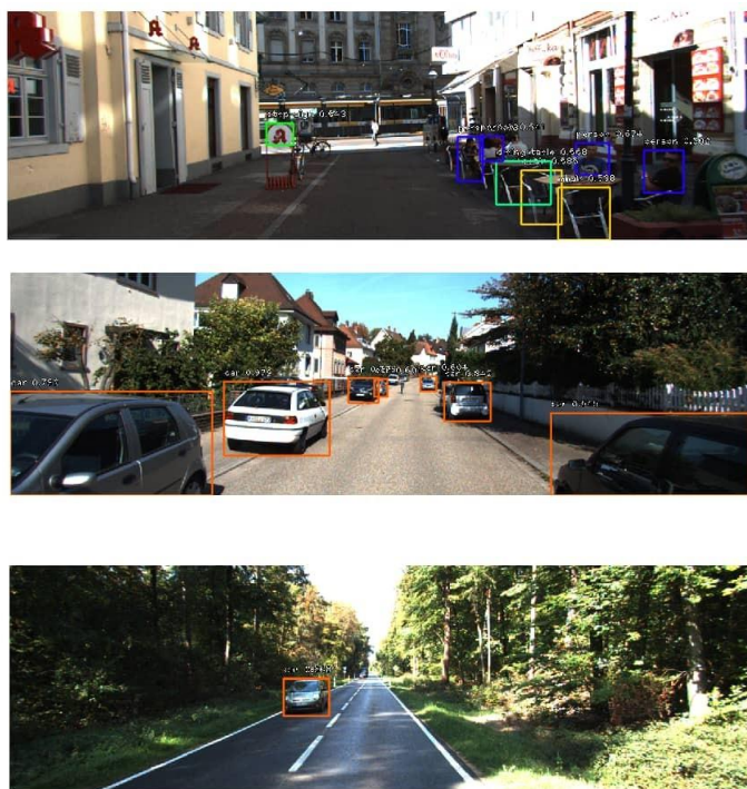
Figure 15: Obstacle detection on the KITTI data using the Unet algorithm
