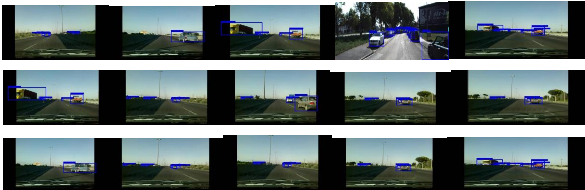
Figure 17: Obstacle detection has also been done using the YOLOv3 algorithm on the images obtained from real driving
