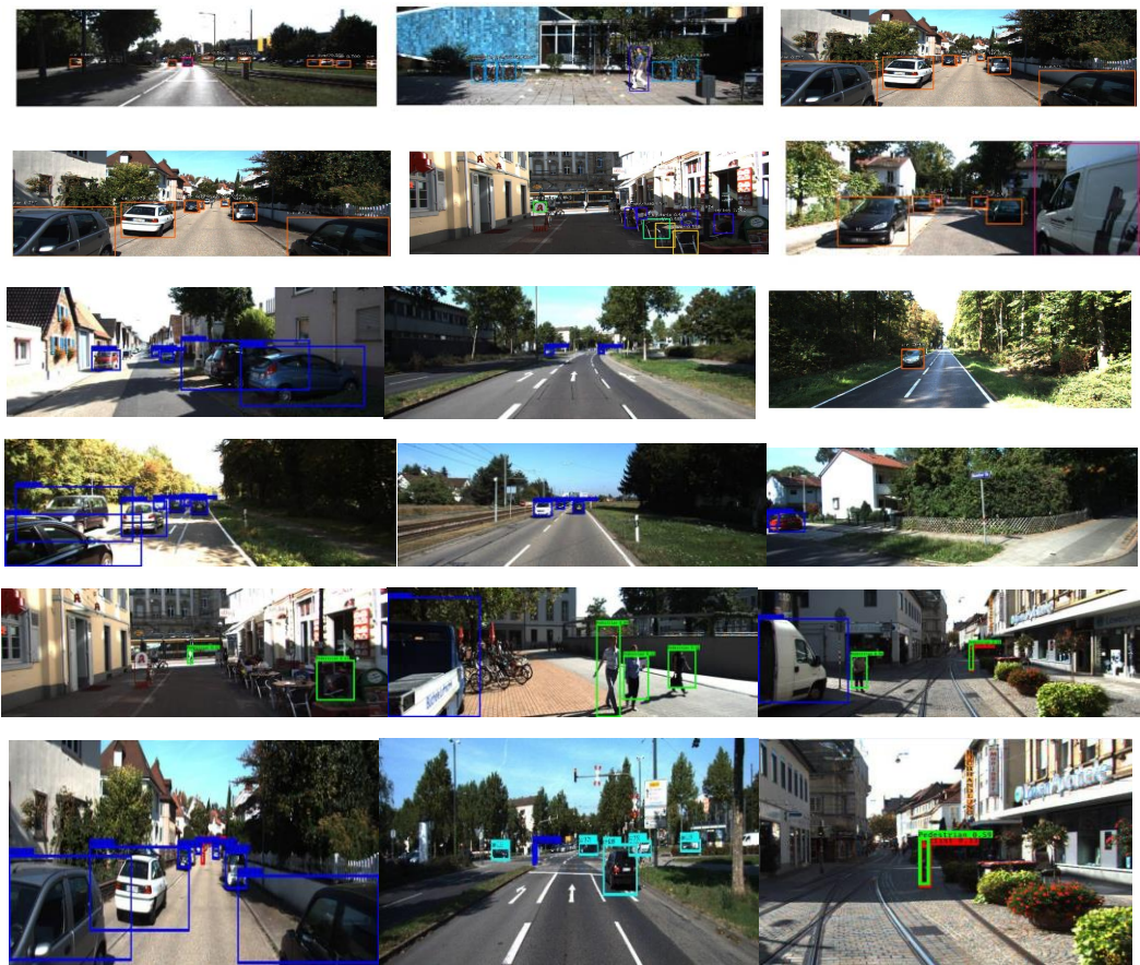
Figure 16: Obstacle detection on the KITTI data using the Resnet algorithm
