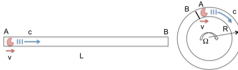
Figure 8: The equivalence of the relative durations the wave takes to propagate a relative distance L , while the frame is moving at the velocity v , for the linear case (left) and for the looped circular case (right). Here, 2\pi R = L , and R\Omega = v . The experiment on the left is not feasible, because the waves would be far from the observer, at the end B, where another synchronized clock is required. The one on the right is the Sagnac experiment.
